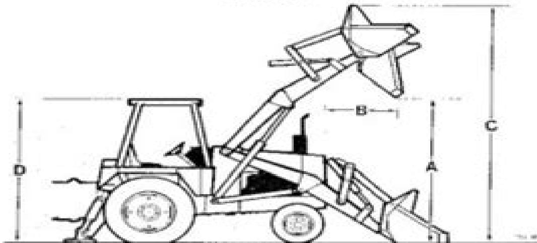
**NOTE:** Specifications taken with 74" (1880 mm) short lip loader bucket, 14.9 x 24 - 6PR rear tires and 7.50 x 16 - 10 PR front tires.
