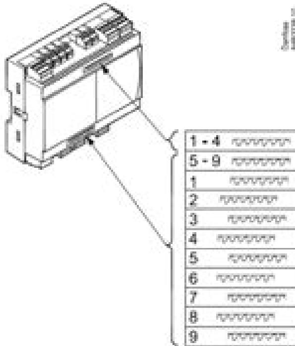
The controller is provided with labels from the factory indicating a general application. When selecting the required application, specific labels are provided so that you can mount the relevant one.
