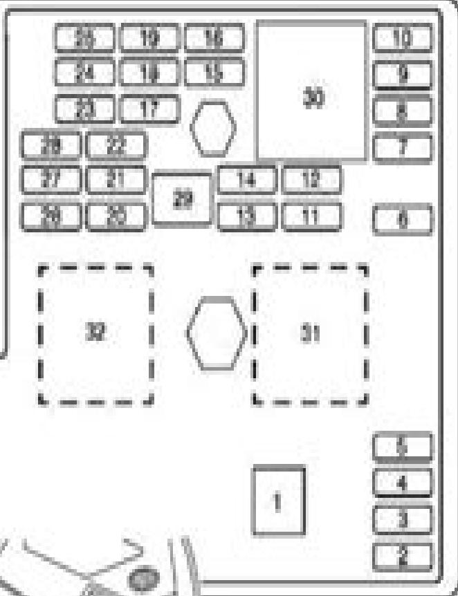
The floor console fuse block is located on the passenger side of the floor console behind the forward panel. The panel has four clips, one in each corner. Pull the panel to disconnect the four clips, and access the fuses.
