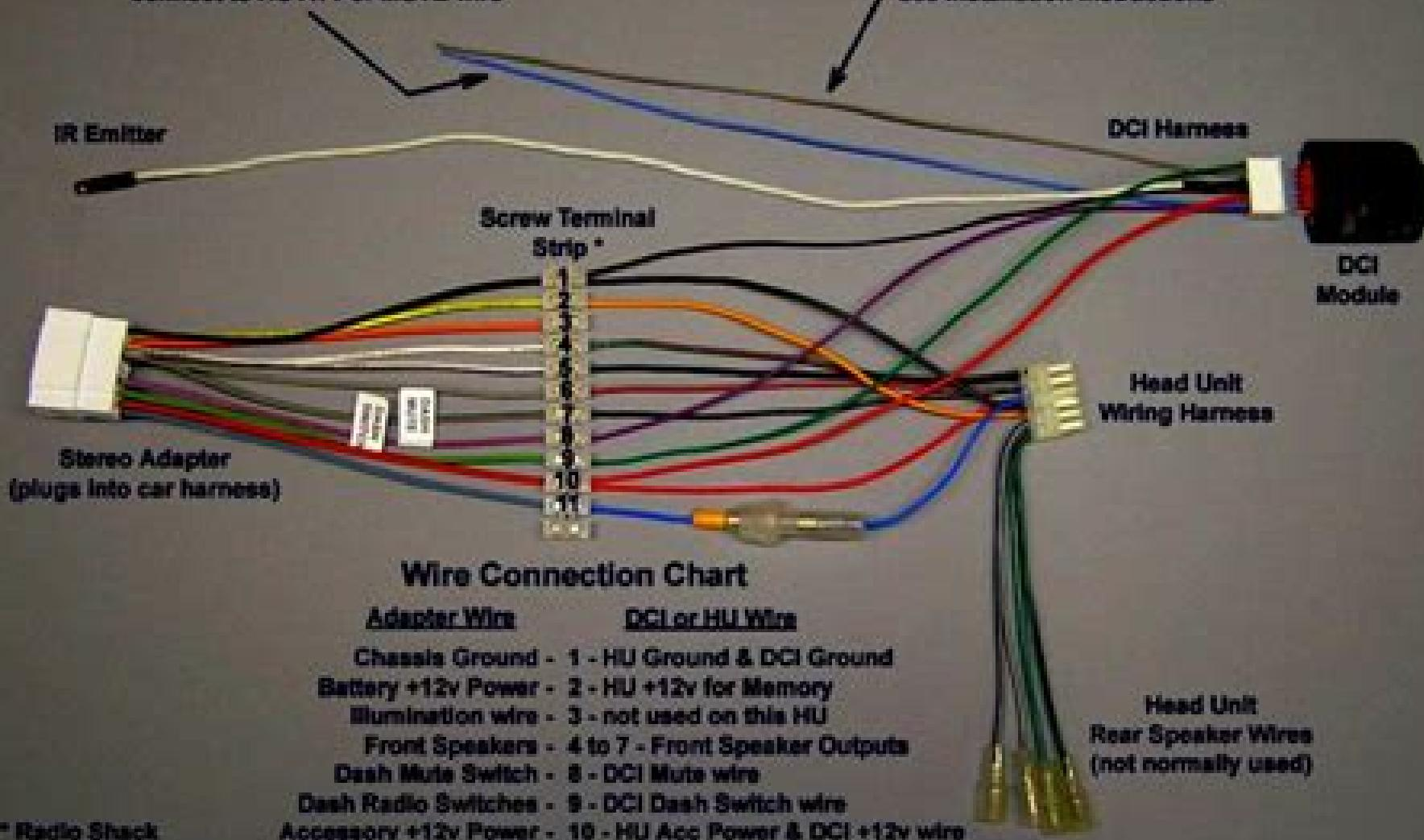
Note: This drawing shows an IR DCI, but the wiring is similar for all types of DCIs. Different HU brands may have different wire colors on the HU Wire Harness, so check your head unit manual before wiring.
