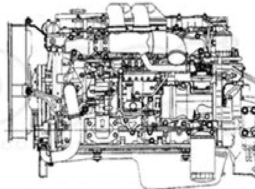
*Diesel L6 / Direct Injection / 8,226 cm<sup>3</sup> / 2 Valve / OHC*
