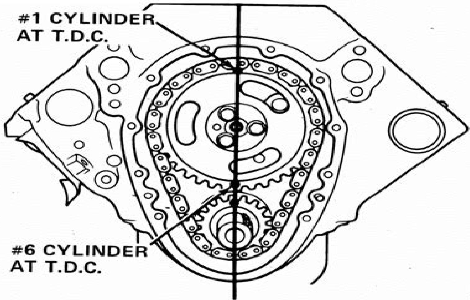
remember the timing or cams gear rotates at 1/2 the speed of the crank gear, thus the crank gear rotates to the 12 o'clock location, once while the #1 cylinder is on its compression stroke, where both gears indicate 12, o'clock or strait up, and once when the #6 cylinder is on its compression stroke, where the timing gear is 180 degrees further, in its rotation where the crank gears at 12 o'clock and the cam gears at 6 o'clock.
