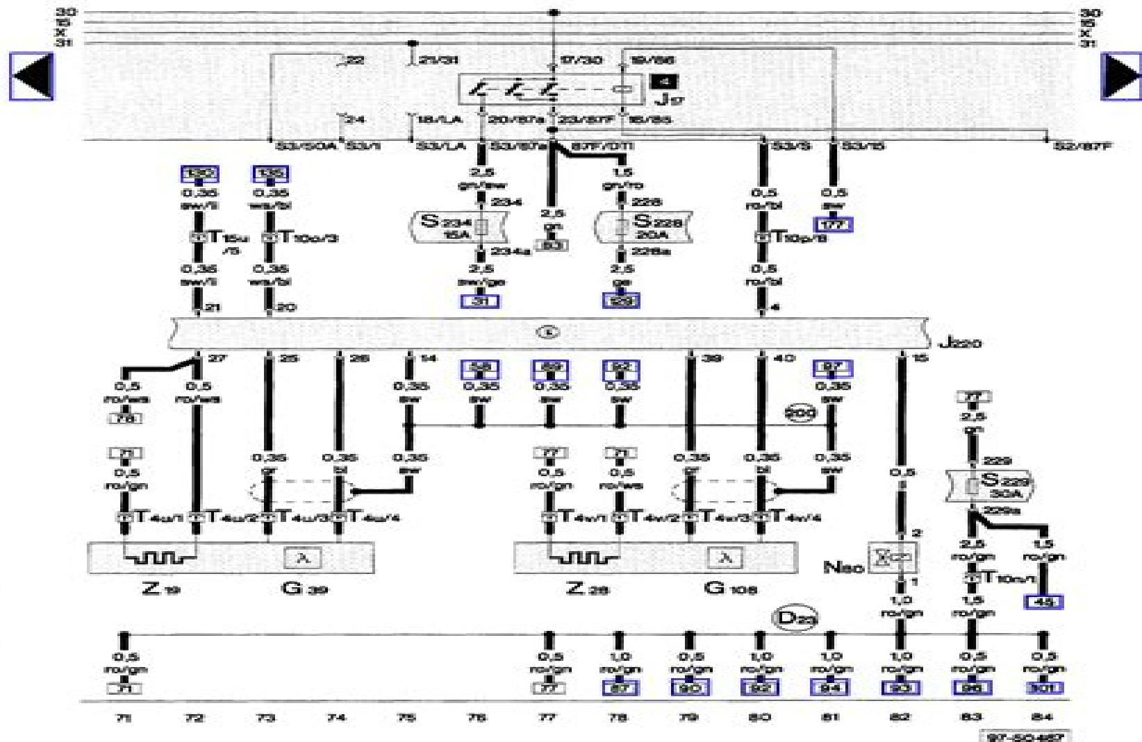
G 39: - Heated Oxygen Sensor (HO2S)
