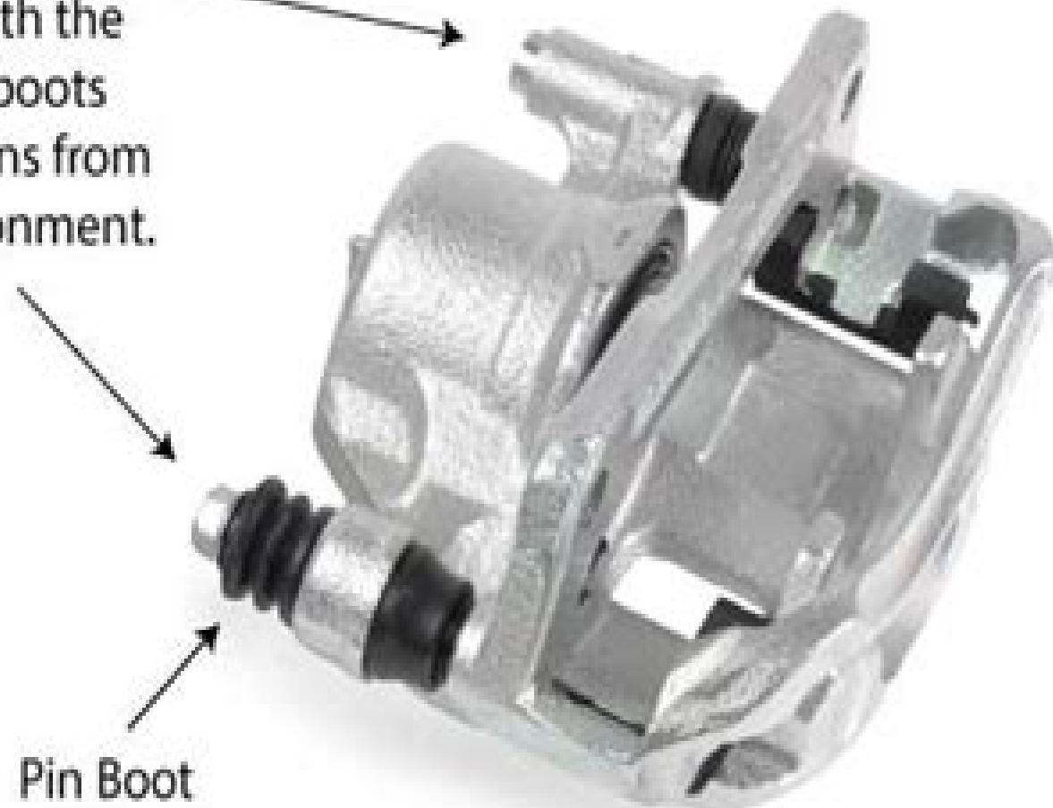
*Disc Brake Caliper*
