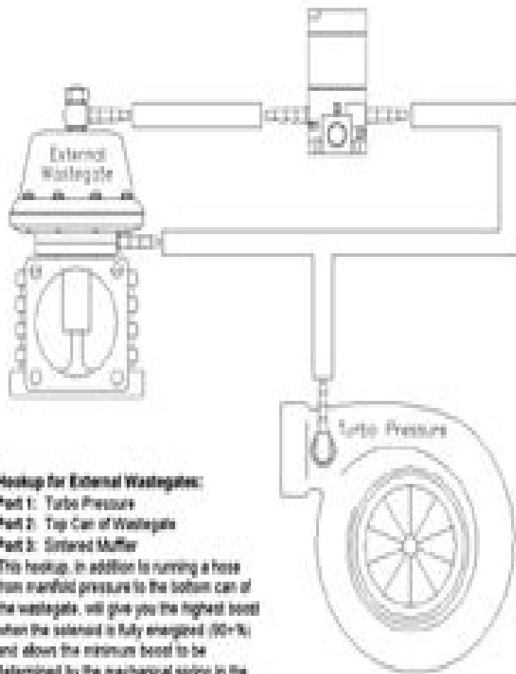
Figure 7. External Wastegate Connection
