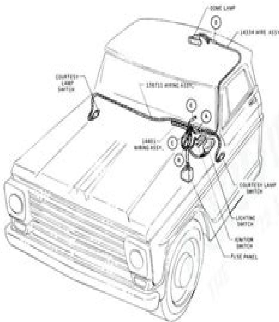
1967 F-100 AND 250 SERIES TRUCK COURTESY LIGHT WIRING
