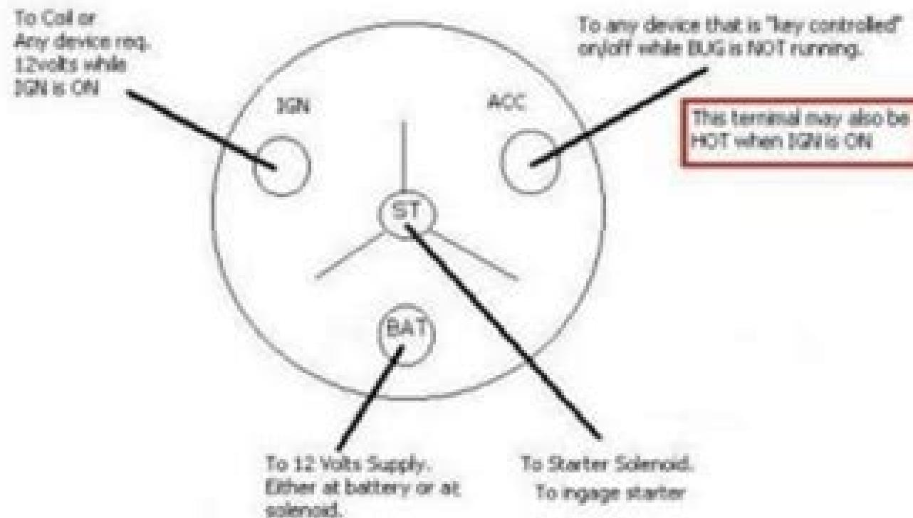
Back side of generic ignition switch. It does not matter where the terminals are physically located on back of switch. What matters is that the designation of the terminal, matches the function one is trying to use it for.
