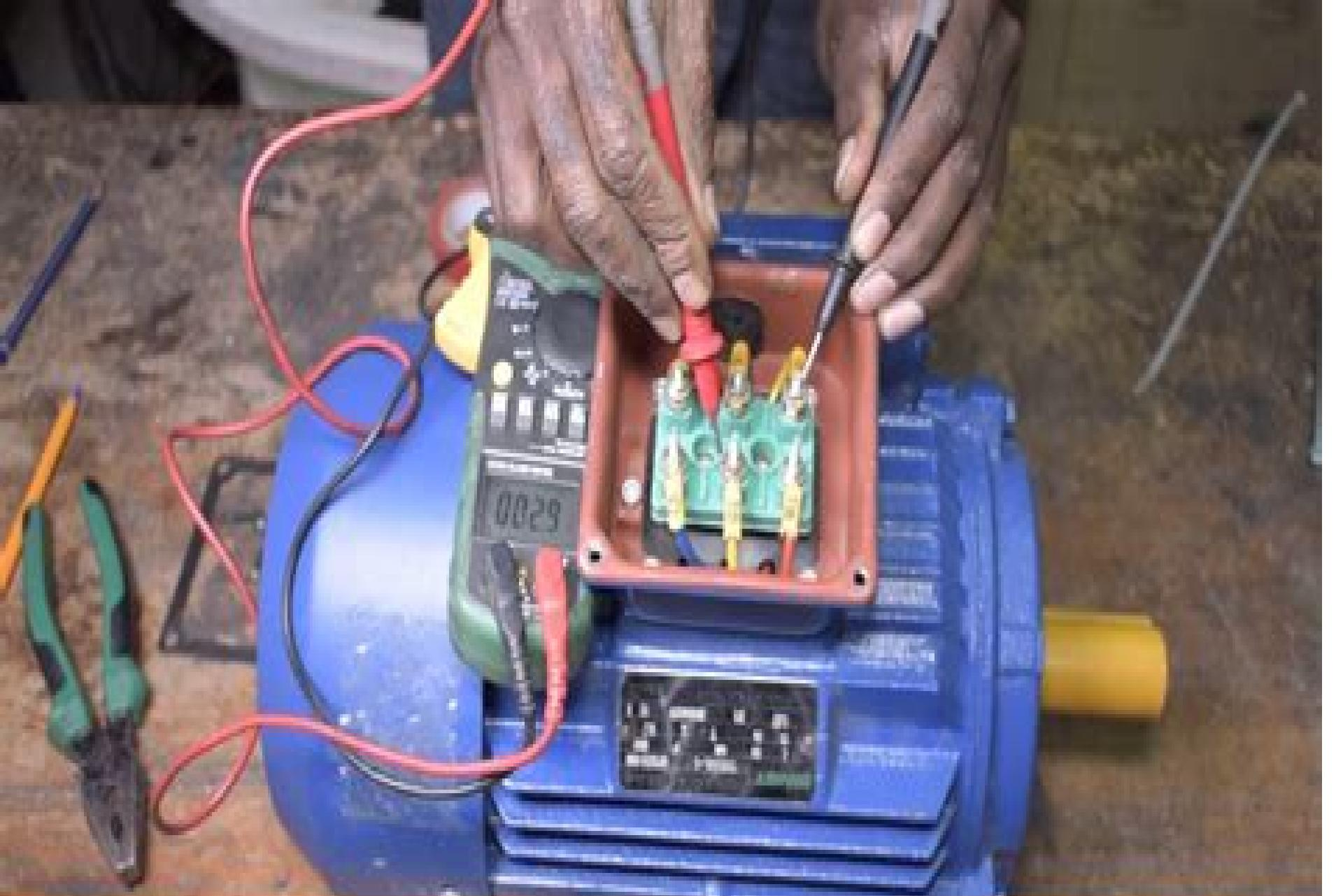
TESTIN 3PHASE MOTOR WITH MULTIMETER
