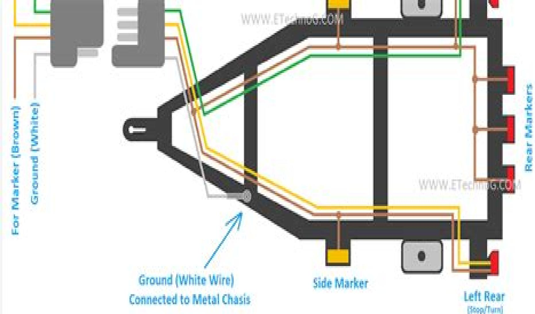
4 Pin/Wire/Way Trailer Wiring Diagram (with Light)
