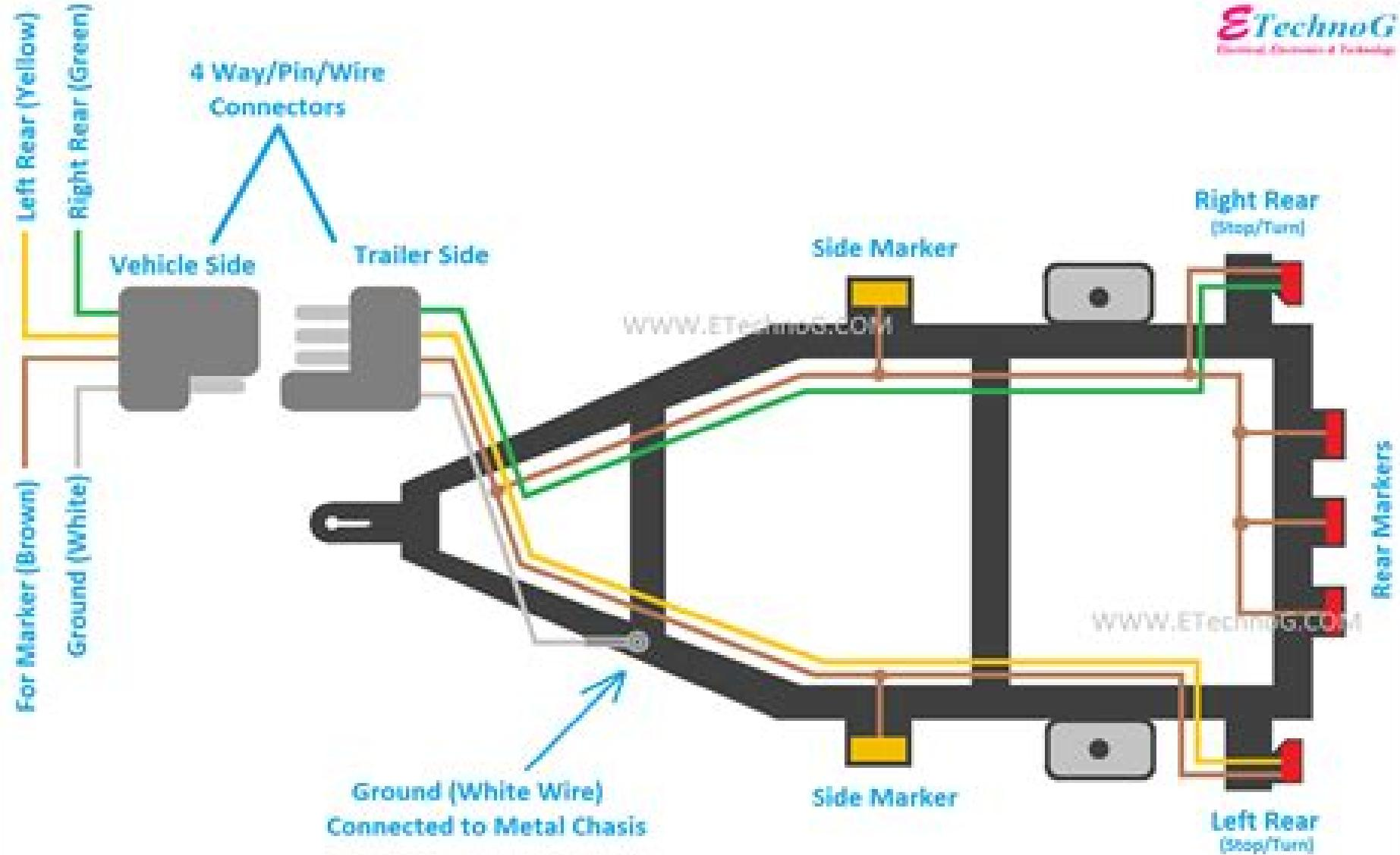
**4 Pin/Wire/Way Trailer Wiring Diagram (with Light)**
