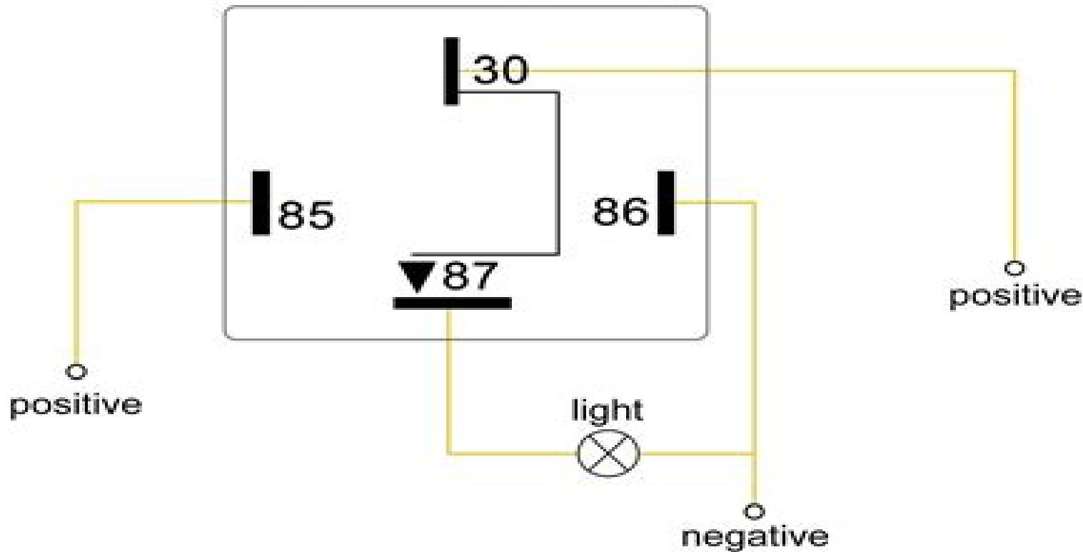
**85** and **86** are the relay coil ends, **30** and **87** are the normally open contact terminals of the relay, when **85** and **86** connect the power, **30** and **87** will be connected.
