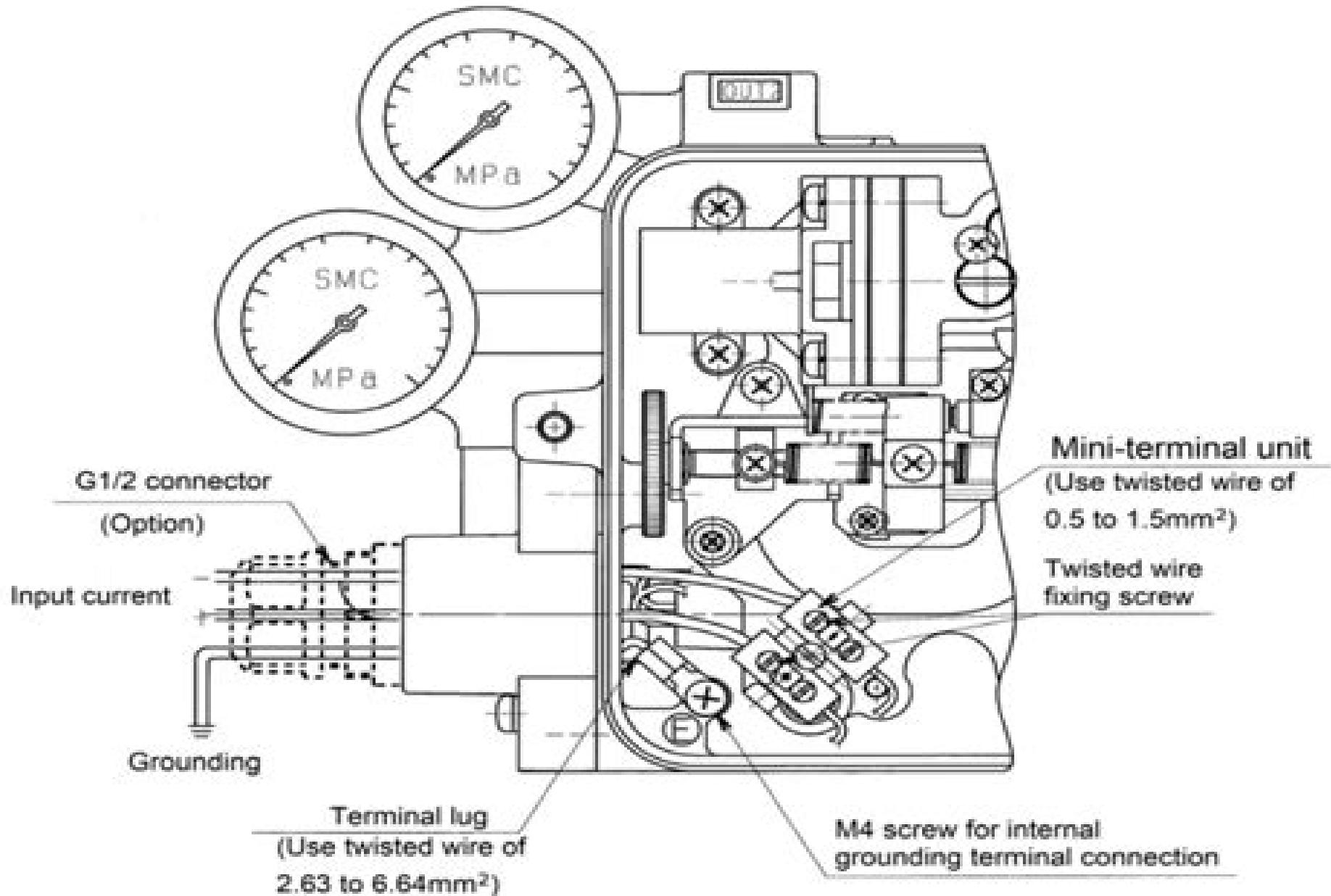
Fig. 15 Positioner without terminal box
