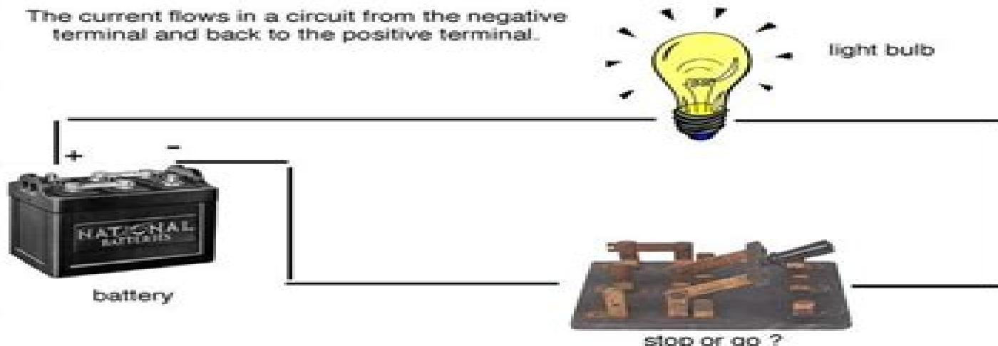
The switch acts like a traffic signal. When the switch is open, there can be no current flow because the road from the negative terminal to the positive terminal is broken. This is called an open circuit.
