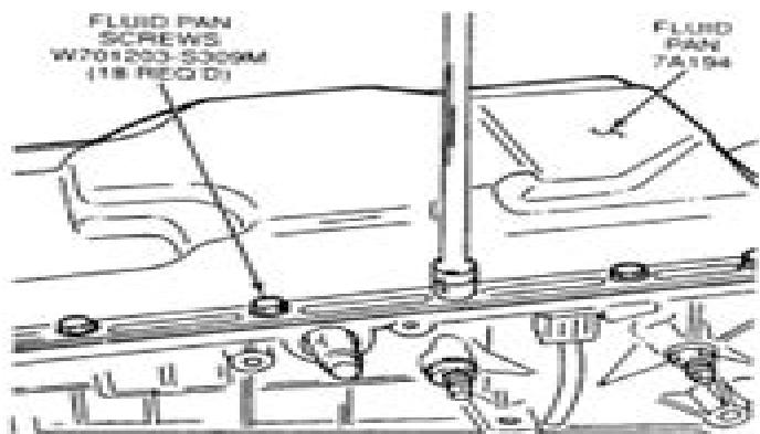
19. Use a 10mm socket to remove the M6 x 5.5mm fluid pan filter assembly screw. Remove the fluid pan filter assembly.
