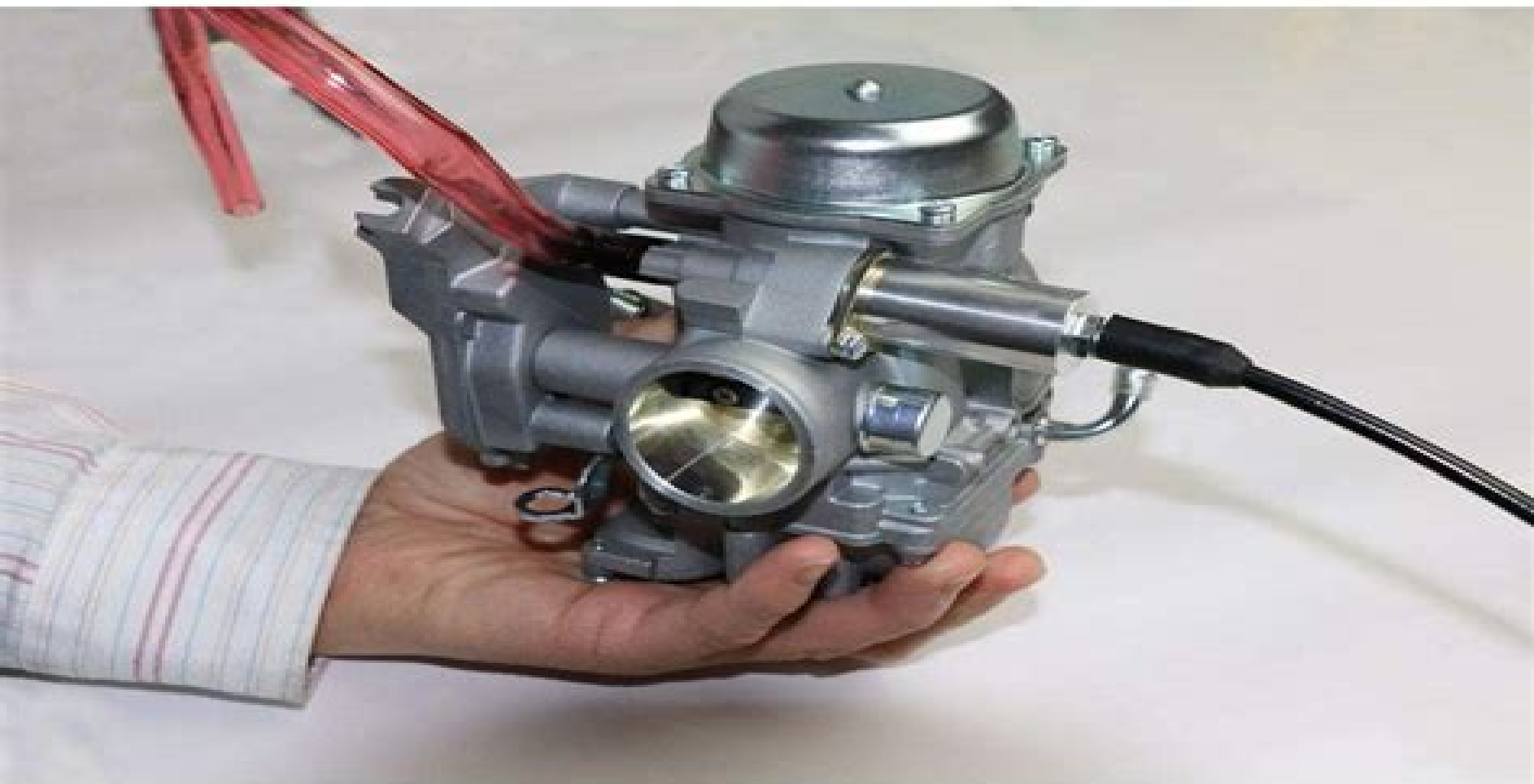
Manual Choke System(After Conversion)
