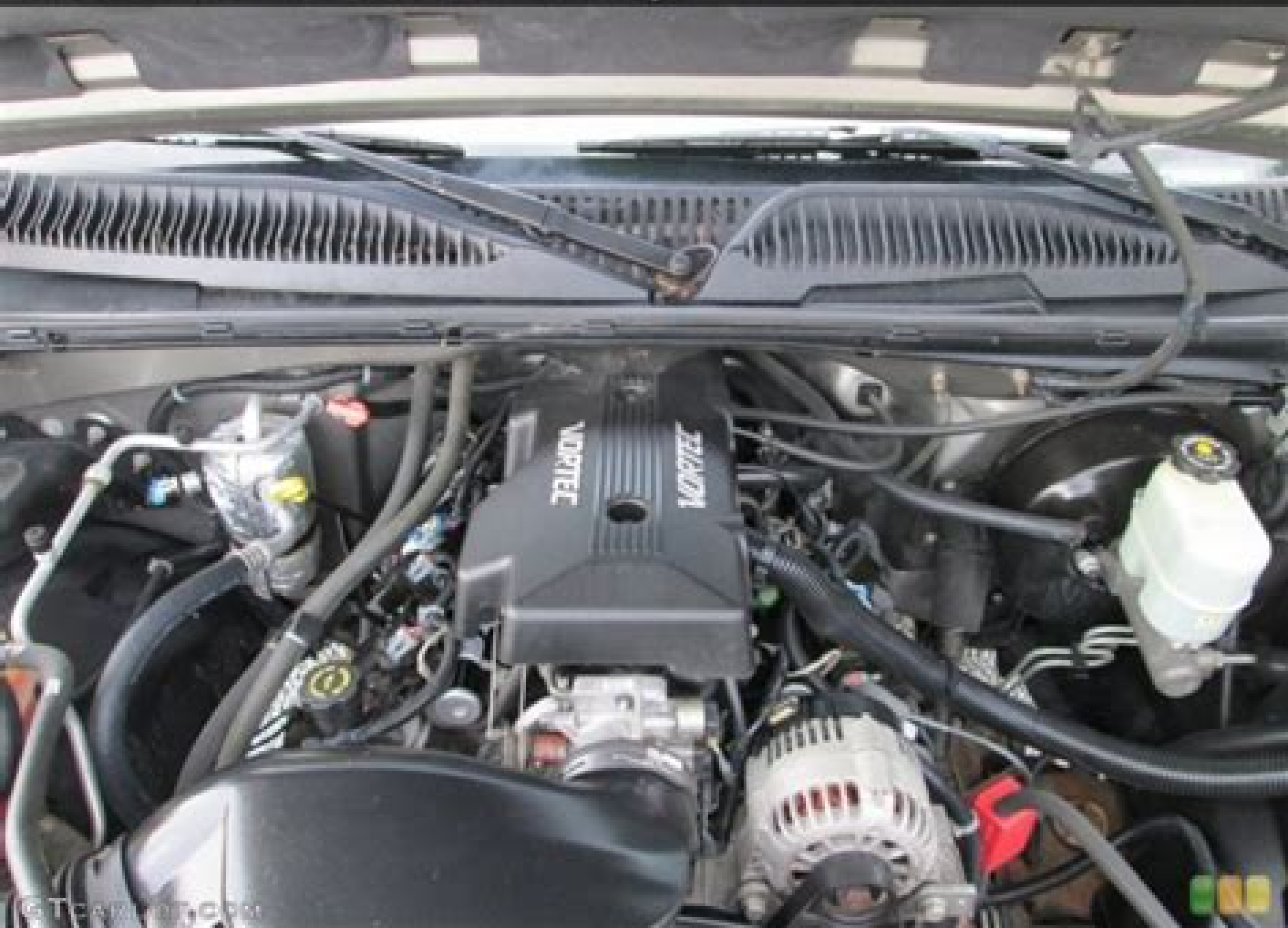
2000 GMC Sierra 1500 SL Extended Cab - 5.3 Liter GMV 16-Valve Vortec V8 Engine
