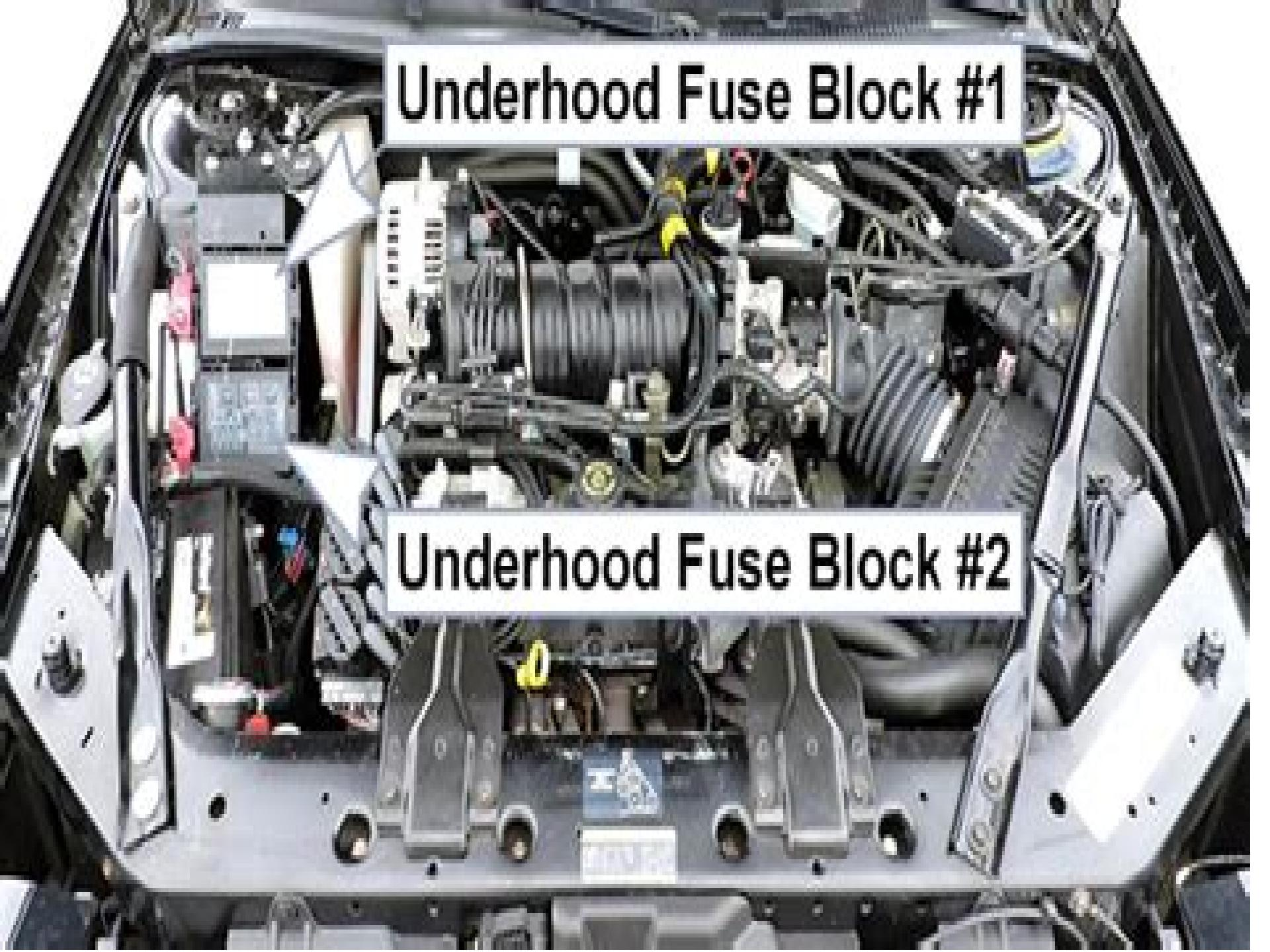
A photograph of the engine compartment of a car. The hood is open, revealing the engine and various mechanical components. Two white rectangular labels with black text are overlaid on the image. The top label is positioned in the upper left area, and the bottom label is positioned in the lower center area. Both labels contain the text "Underhood Fuse Block #1" and "Underhood Fuse Block #2" respectively. The labels are semi-transparent, allowing the underlying engine components to be seen.
