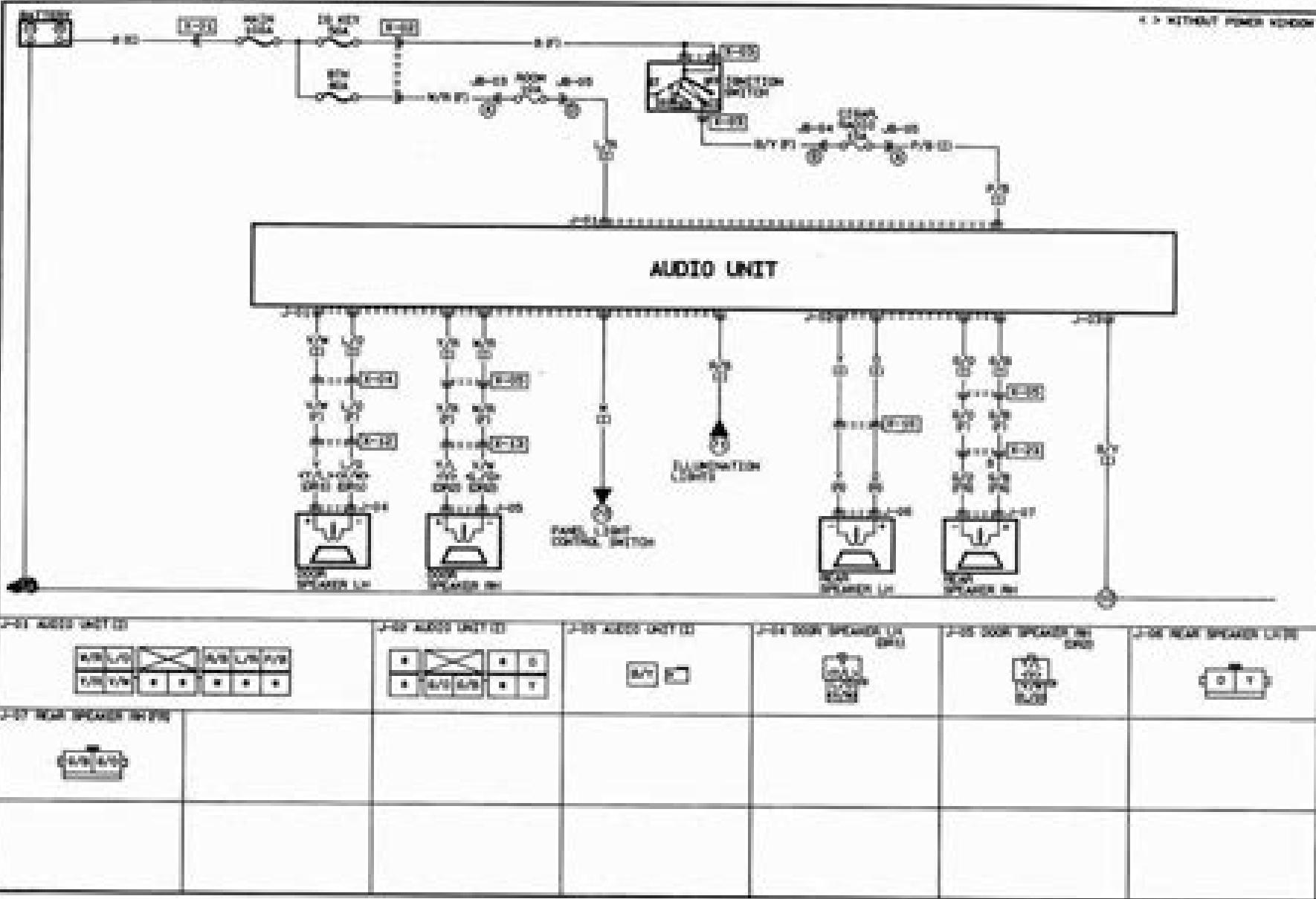
Wiring diagram for radio and speakers - 1997 model shown (typical for 1996 and later)
