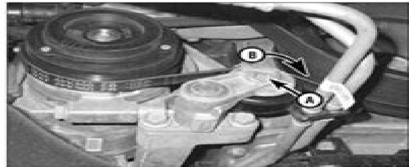
12.5b On V8 models with air conditioning, the inner belt tensioner is best accessed from below - use a 3/8-inch-drive tool in the tensioner's square hole (A) to rotate it (B) for belt removal
