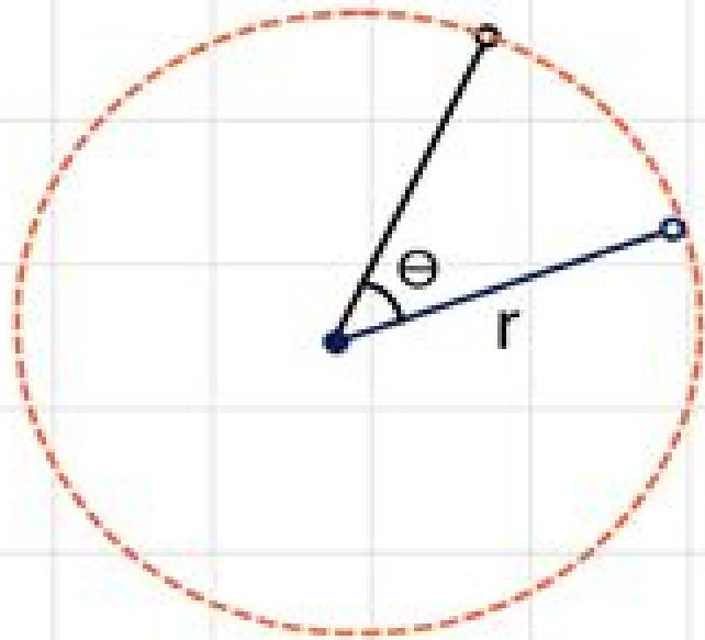
$$\text{arc length} = \frac{\theta}{360^\circ} \times 2\pi r$$
