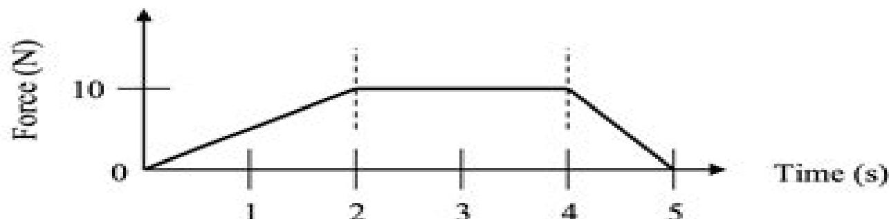
An object of mass  $m = 2.0\text{kg}$  experiences a force in Newtons according to the *Force vs. time* graph shown here. For the time interval shown, what is the total change in momentum of the object?
