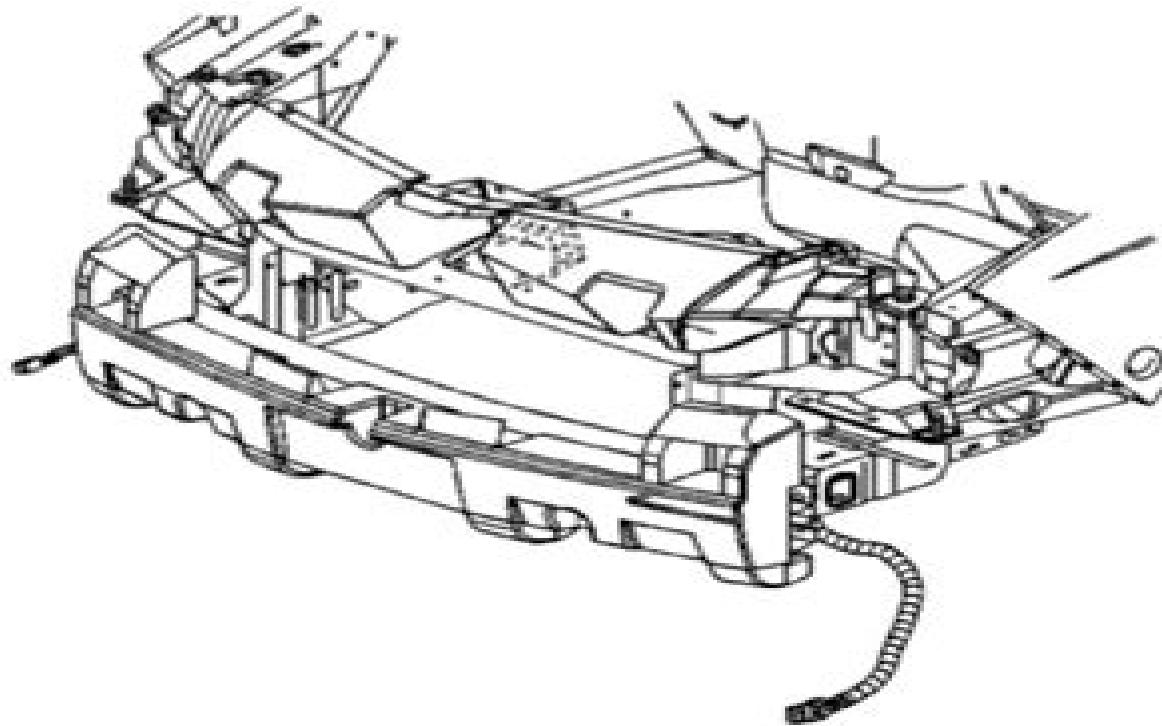
**Fig. 38: View Of Headlamp Wiring Harness**
