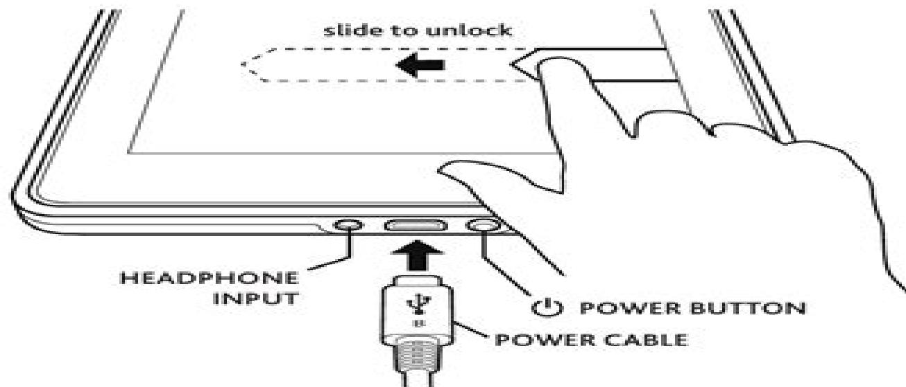
To charge your Kindle, connect it to the power cable as shown. Then connect the power adapter at the opposite end of the power cable into a wall outlet.
