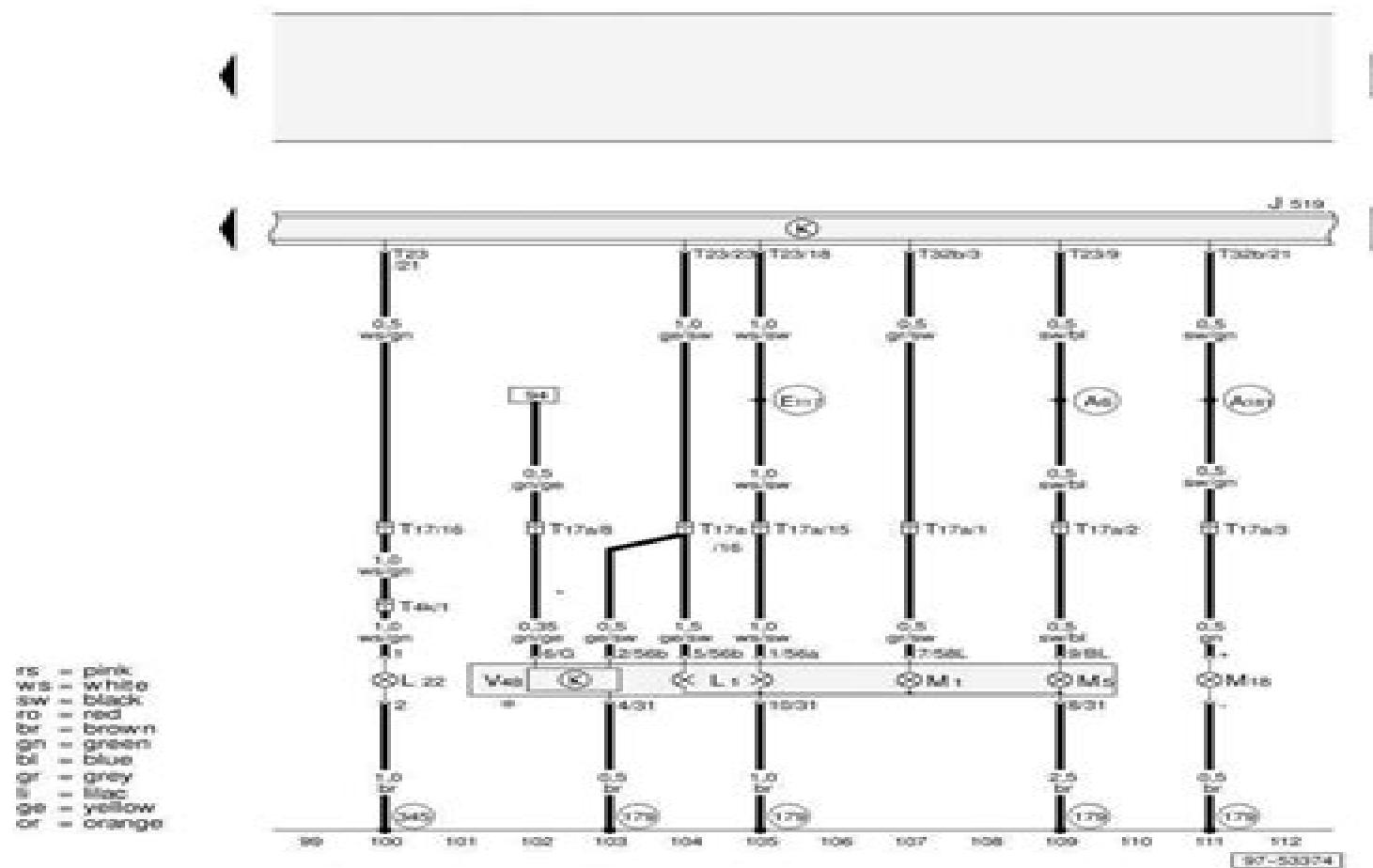
JS19 - Vehicle Electrical System Control Module
