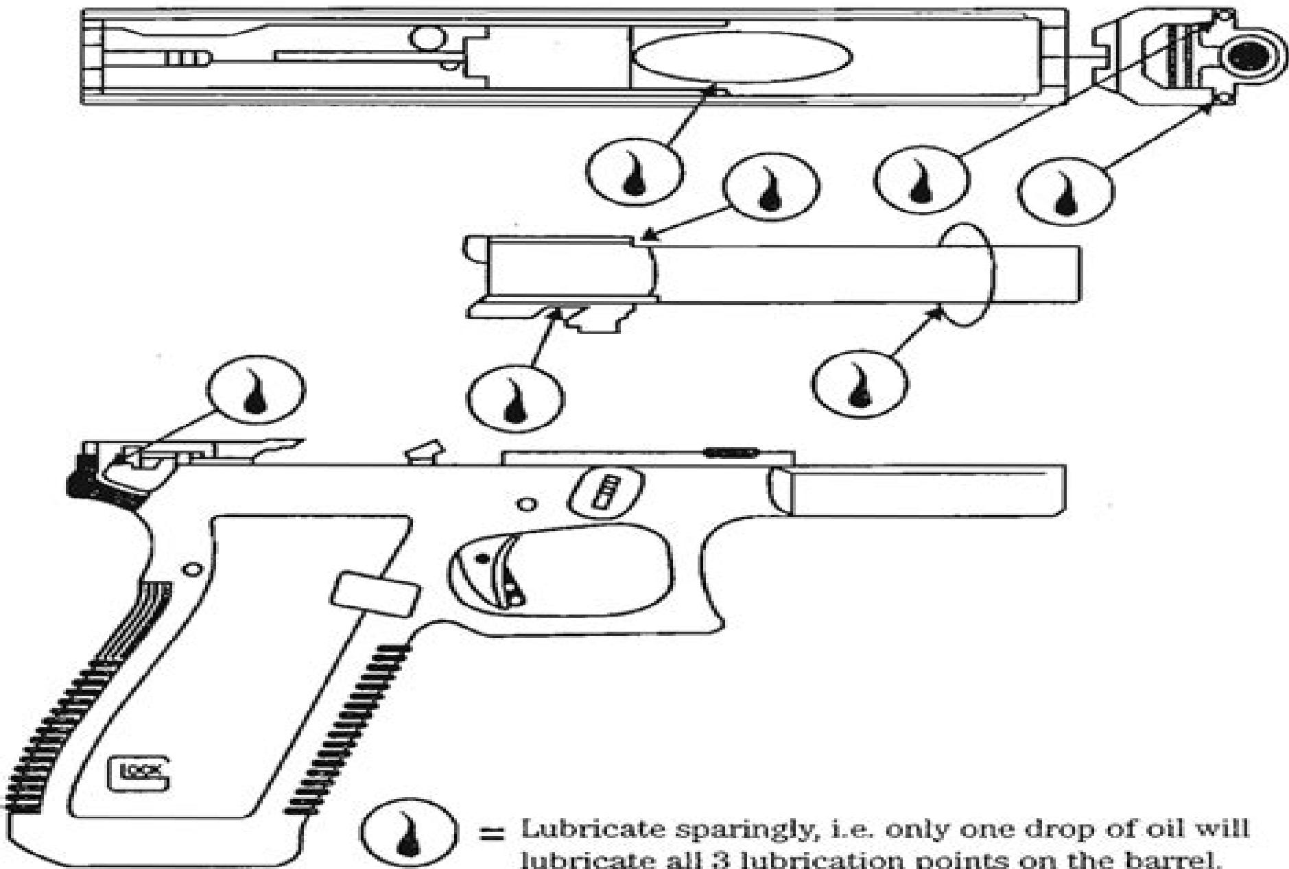
= Lubricate sparingly, i.e. only one drop of oil will lubricate all 3 lubrication points on the barrel.
