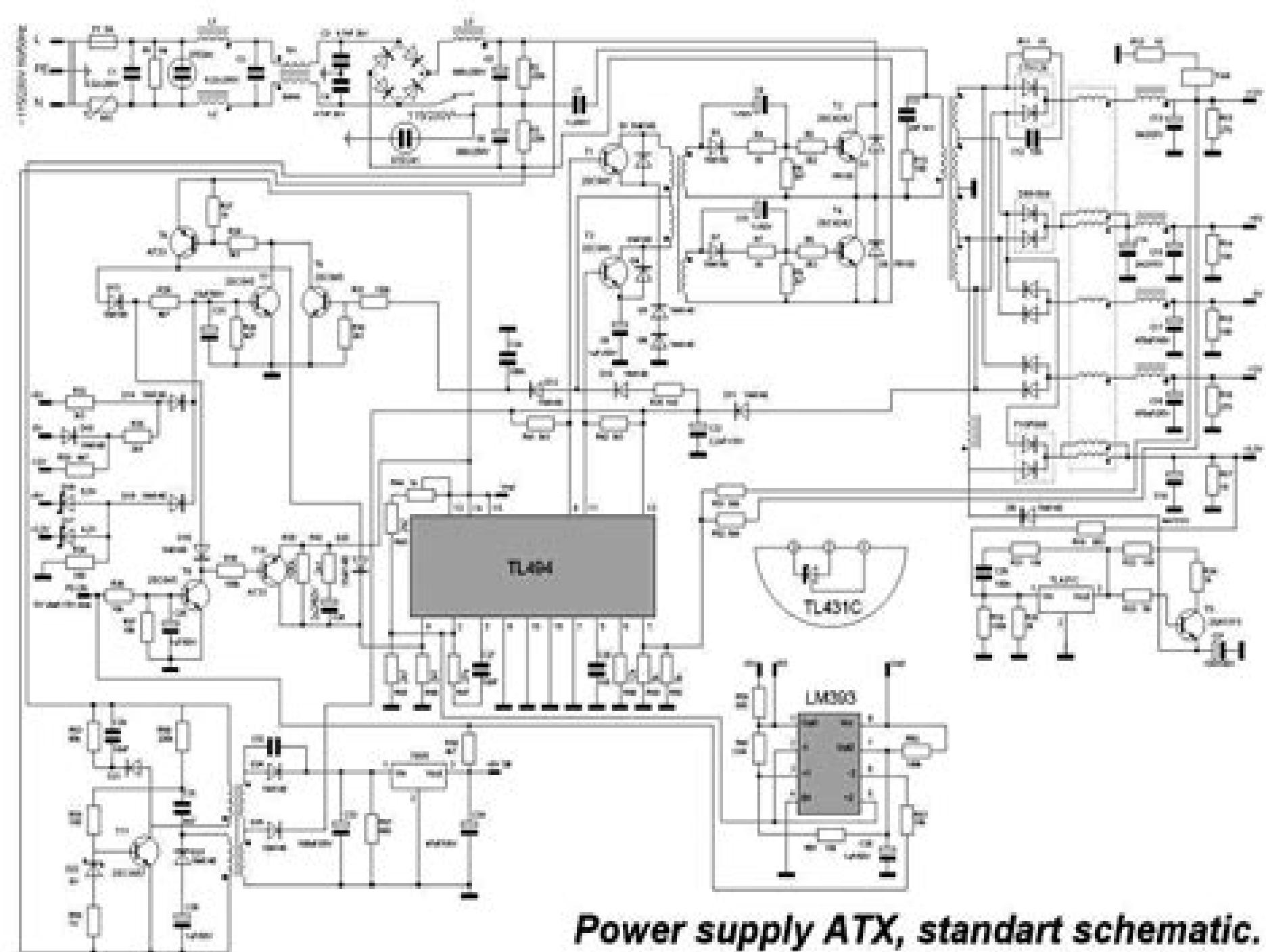
*Power supply ATX, standart schematic.*
