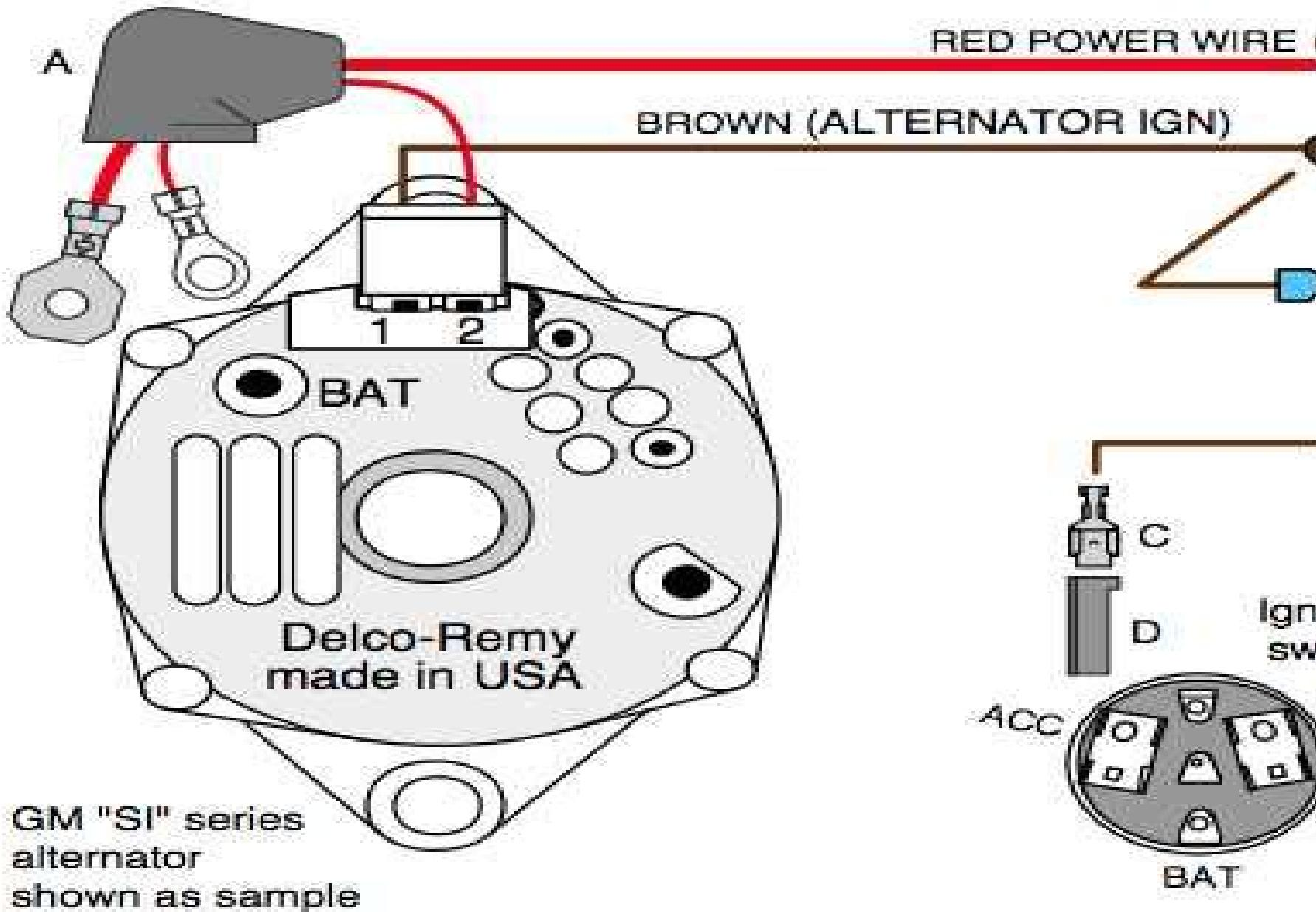
Our Highway 22 instruction sheet illustrates the exciter wire (brown, alternator ign) used for a GM SI-series alternator. This is not needed with a one-wire alternator.
